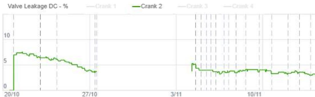
Figure 7. Crank 2 CE discharge valve leakage trend line
