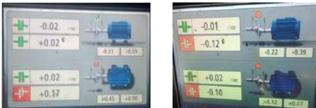
Figure 7: Correction of alignment in Trial 1
