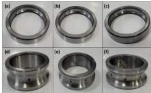
**Fig. 3. Single and multiple defects on bearing races (a) single defect on OR (b) two defects on OR (c) three defects on OR (d) single defect on IR (e) two defects on IR (f) three defects on IR.**
