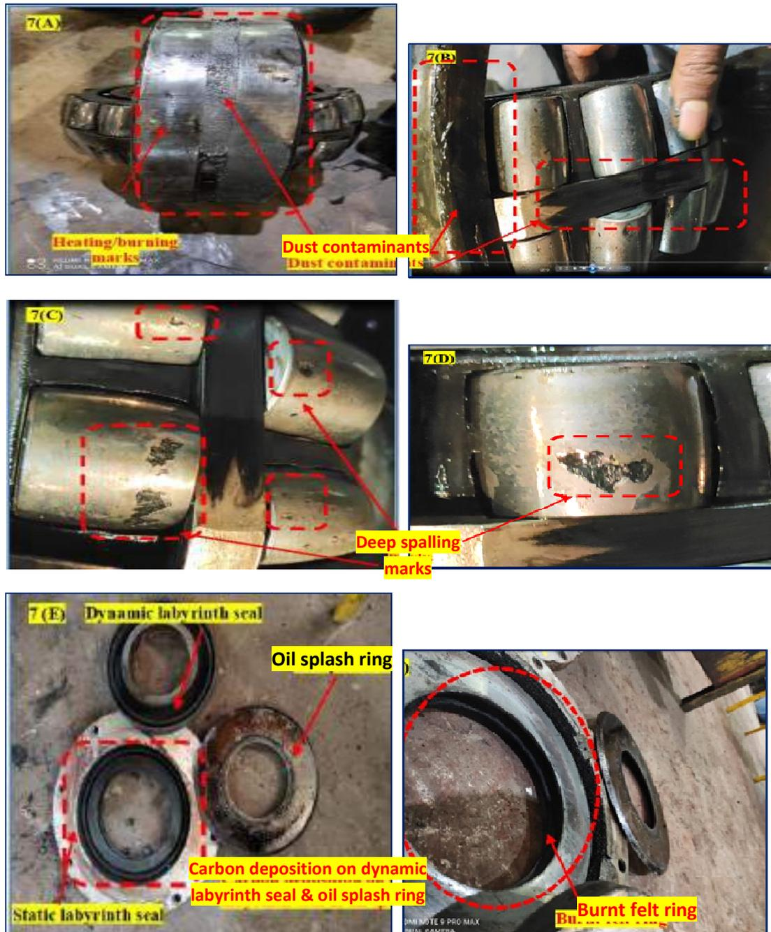
Fig.-7 Failed bearing
