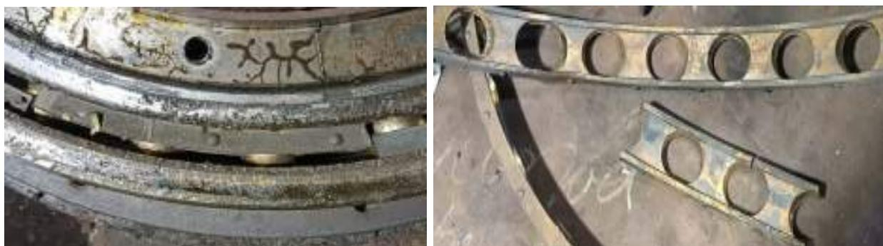
Figure:11 Broken cage of the failed bearing found after dismantling
