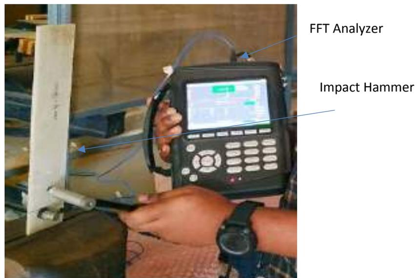
Fig. 2 Impact hammer test on cracked composite beam
