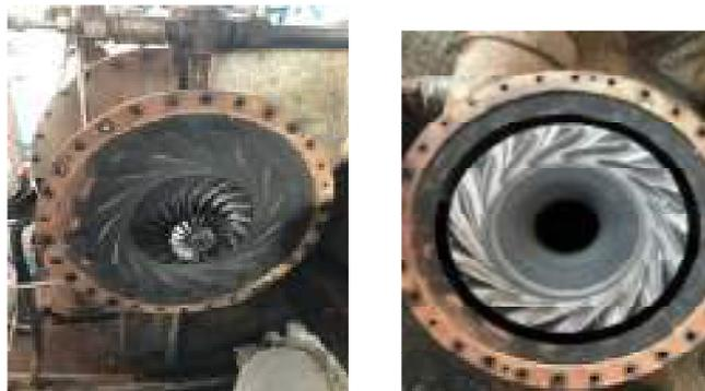
Fig 2: Dust accumulated on Impeller and diffuser of 150KM2A compressor
