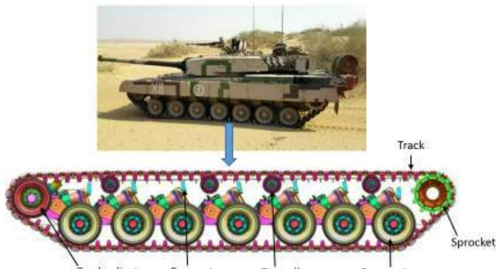
**Fig.3. Running gear system for Main Battle Tank**
