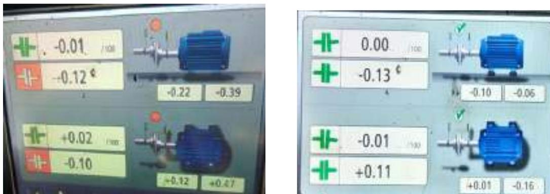
Figure 9: Correction of alignment in Trial 2
