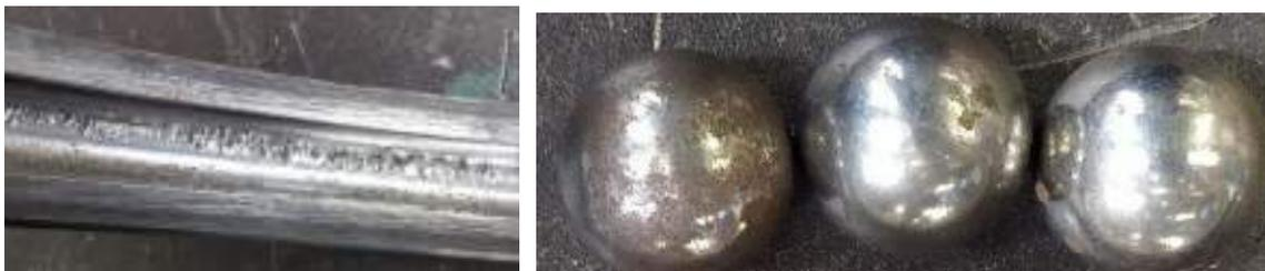
Figure: 13 Damaged inner race and the rolling elements of the failed head pulley bearing
