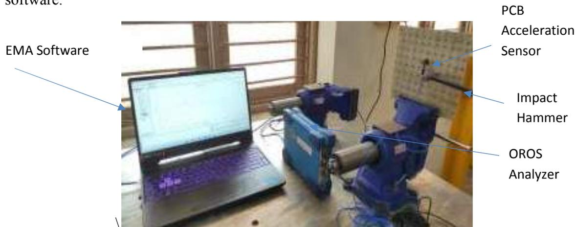
Fig. 2 Image of experimental modal analysis setup
