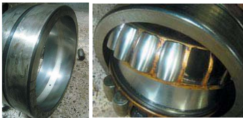
Defective Bearing Shows Signs of Severe Wear
