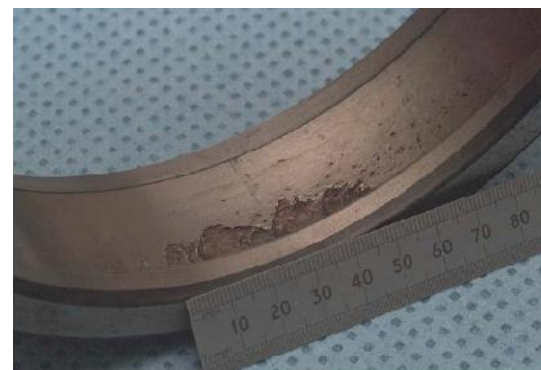
Fig.4 Photograph showing bearing outer race damage
